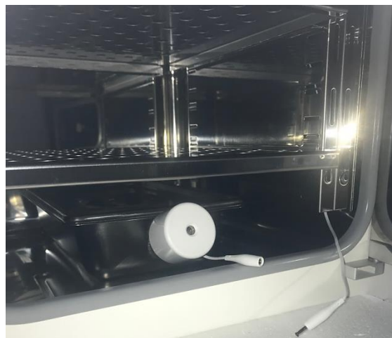
#2. Disconnecting the cable before taking tray out
