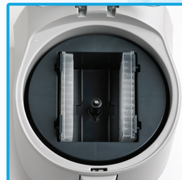
Horizontal Rotor Position (During Centrifugation)
