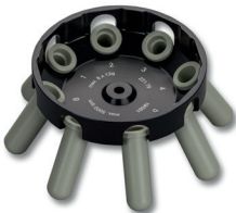
max. volume: 8 x 10 blood tubes Order number.: Z287-0810H
