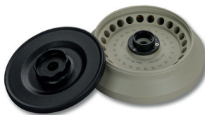
max. volume: 24 x 1,5/2,0 ml Order number.: Z287-2420H hermetically sealed
