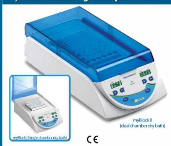
Benchmark's myBlock<sup>™</sup> series are the first digital dry baths to include advanced microprocessor controls, timed operation and a removable, hinged lid. In addition, an optional external temperature feedback probe can be positioned directly inside a sample tube, providing real-time control and monitoring of actual sample temperature.
