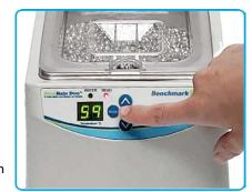
The BeadBath Duo series is the first line of laboratory baths designed for precision temperature control when used with water, or with the increasingly popular Lab Armor® thermal beads.
