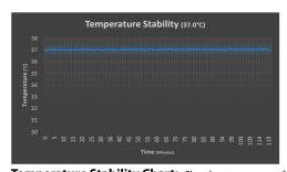
**Temperature Stability Chart:** Chamber temperature for a 2 hour duration following stabilization (within 0.1 °C) at 37.0 °C.
