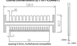
Large teeth: 5.65x1mm, well volume 22.6µl for 0.5mm thick gel Small teeth: 3x1mm, well volume 12µl for 0.5cm thick gel 3mm wide teeth taper from 2mm to 1mm at tip
