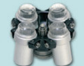
Z326-100H 4 x 100ml Swing out rotor with buckets 4,500 rpm/ 2,716 xg
