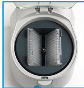
Before & after centrifugation (angled position)
