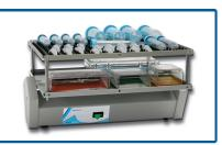
The **BenchBlotter** is the first rocker to be specifically optimized with the ideal rocking speed and tilt angle for blot washing, gel staining/destaining and hybridization applications. Available with an optional dual platform accessory, the **BenchBlotter** offers a sizeable work space, while maintaining a compact footprint and low profile design.
